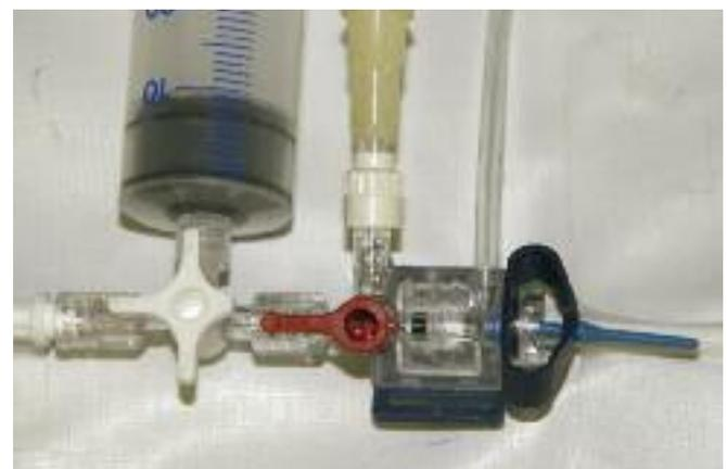
Figure 2. Transducer configuration attached to an air-less intravenous fluid infusion set for measuring pressure ( $P_f$ ).
